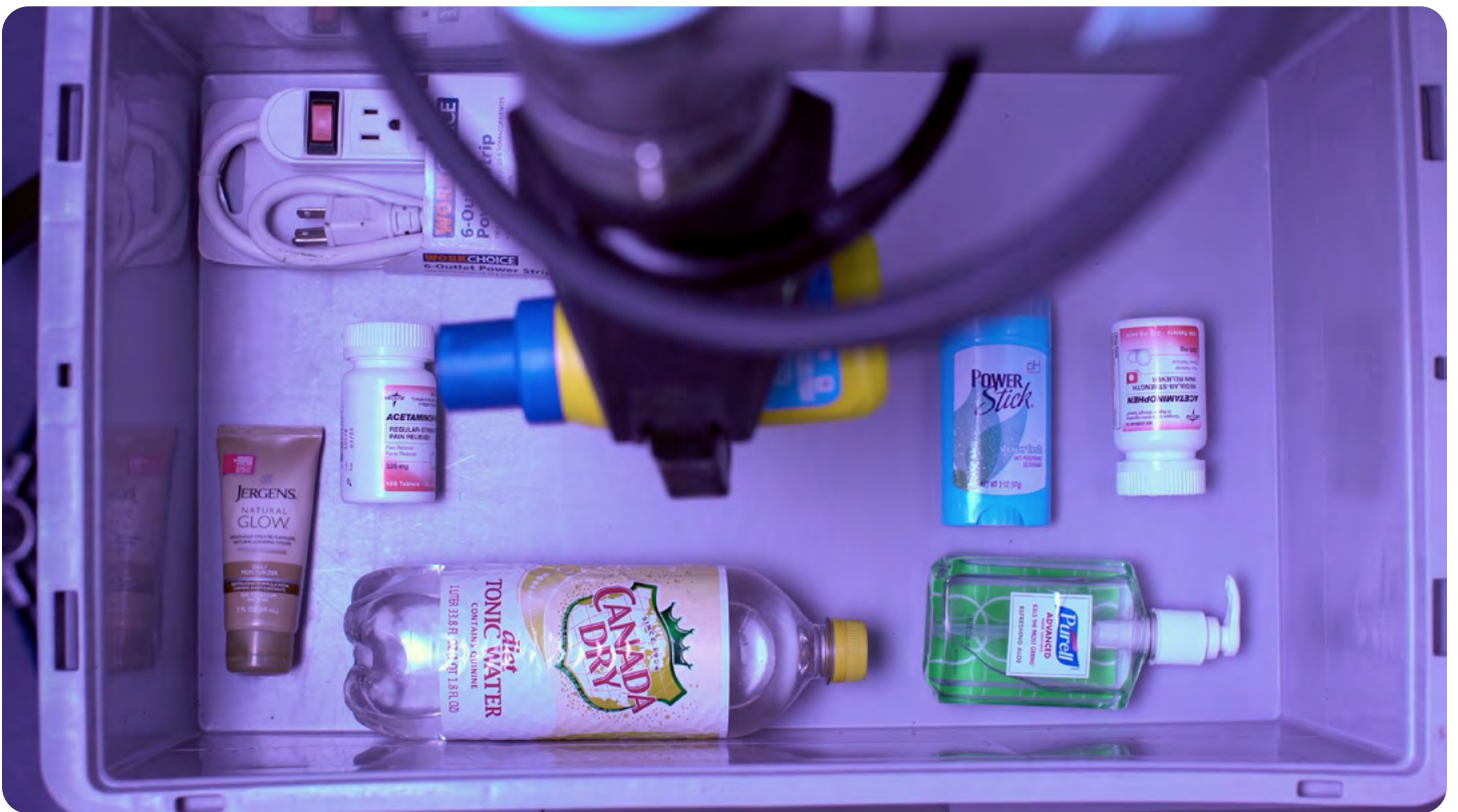
TOP: A gripper uses suction to hold and rotate a product while its barcode is being scanned. BOTTOM: A gripper lifts and removes products of different shapes and sizes from a bin. Stills from videos by Mae Ryan for Aventine.
