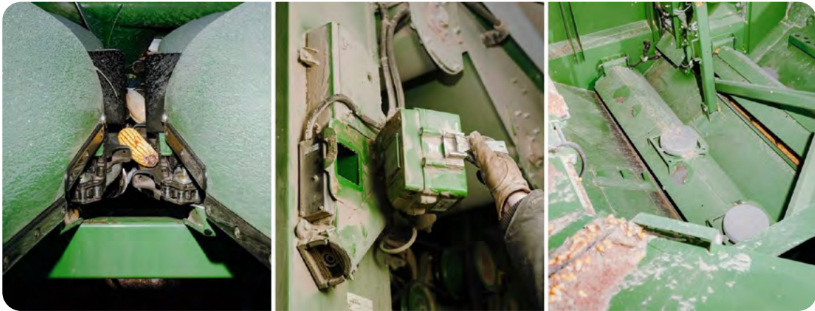
FROM LEFT TO RIGHT: A cob of corn in the combine; a camera that monitors corn as it comes through the grain elevator; load cells (the silver-colored discs) record the quality of the yield as it is being processed. Lyndon French for Aventine
